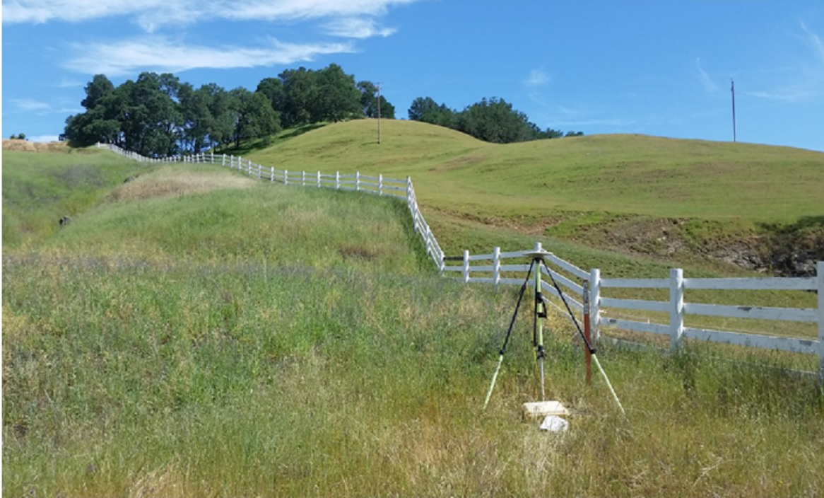
Figure 3 - Global Navigation Satellite System (GNSS) surveys are frequently used for establishing blind checkpoints, but differential levels may be required to establish elevations for the most demanding projects.
